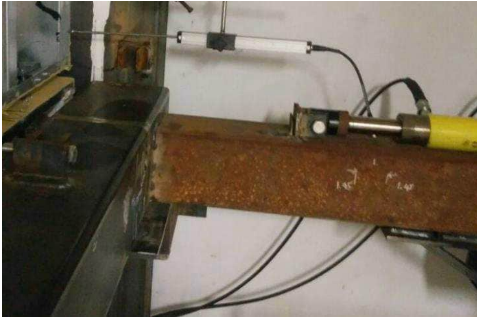
Photo B14: Interstory Horizontal (in/out) movement equipment set-up
