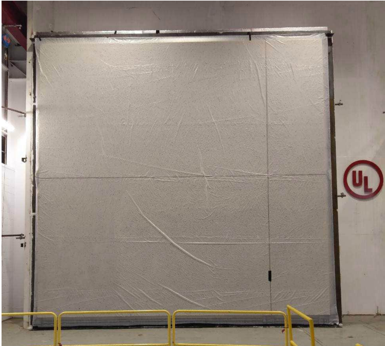
Photo B1: Application of plastic film for the chamber tare (Extraneous Air Leakage)
