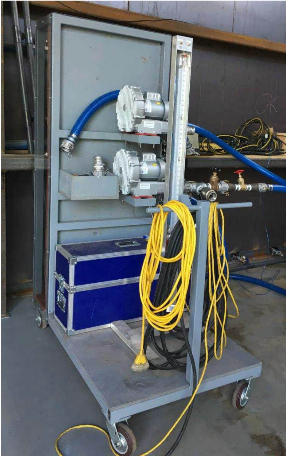
Photo B2: Air infiltration/exfiltration testing equipment
