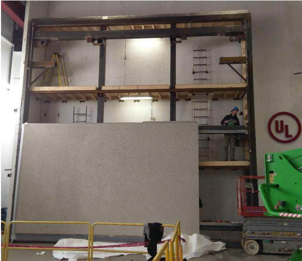
Photo A7: First panel installed onto test chamber
