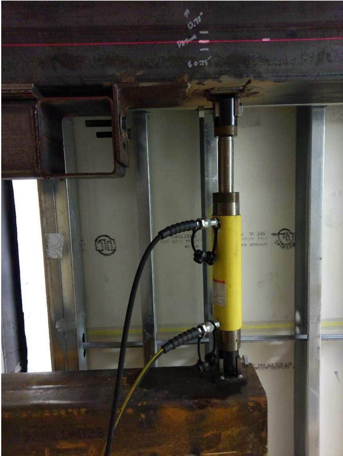
Photo B17: Interstory Vertical (up/down) movement equipment set-up reference datum
