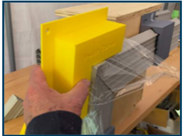
Corner Blocks hold Strong-Back in place until sealant cures
