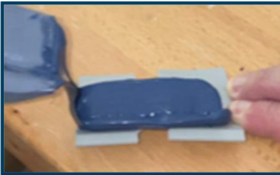
Apply Sealant on Strong-Back
